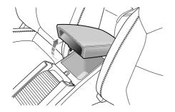
Lift the armrest (arrowed) to open the compartment cover. Put the cover down to close it.
