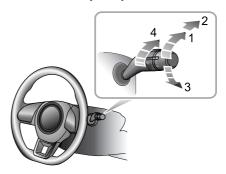
The rear window wiper and washer will only operate with the vehicle power system in the ACC/ON/READY position. Operate the lever to select different wipe speeds:
