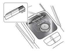
The driver can operate the BATTERY switch backward to display the energy management interface in the infotainment system.
