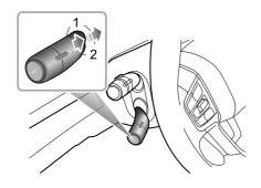
The traffic jam assist system switch is located in the infotainment display. Enter the corresponding interface for driving assistance to turn the system ON/OFF. Operating the adaptive cruise control level to "RESUME" twice will switch the traffic jam assist system into the standby or active state.
