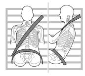
When wearing seat belts, the lap belt section should be positioned as low as possible across your hips, never across the abdomen. In the event of a collision, the lap belt can apply a force on the hips and reduce the possibility of you
