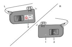
Note: Warnings and instructions on use of child restraint (3) are attached to both sides of the passenger sunvisor.
