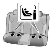
3 To fasten the top tether strap of the child restraint system, route the tether strap under the head restraint and attach to the anchorage hook being careful not to twist the strap. If not using ISOFIX lower anchorages, using the seatbelt, complete the installation in line with the child restraint manufacturers instructions. Note: When using seat mounting, universally approved child restraint systems, Top-tether must be used.
