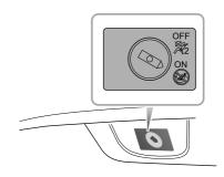
The passenger airbag disable switch is located inside of the glovebox, Insert the key and turn the switch to the on or off position to enable or disable the passenger airbag.
