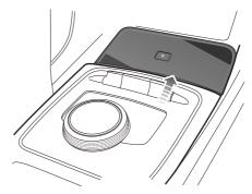
The wireless charging area is located in the area shown in the figure. The charging function is enabled when the START/STOP Switch is placed in the ACC/ON/READY positions. Place the phone face up horizontally in the charging area, which can be used for wireless charging.
