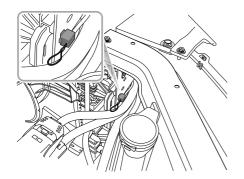
Pull the release cable handle, remove the connector plug whilst maintaining tension on the cable this will release the locking device.
