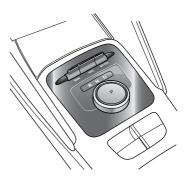
The shift control knob is in the intermediate steady state position, and there are two unsteady positions clockwise and counterclockwise, that is, the shift control knob will return to the intermediate steady state position once released
