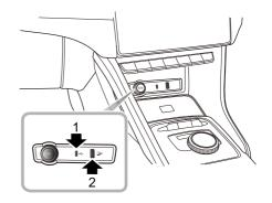
The 12V power socket is located in front of the shift control knob assembly in the centre console. It can be used as a power supply when the START/STOP Switch is in the ACC or ON/READY positions when the blanking plug is removed.
