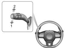
Move the lever down to indicate a LEFT turn (I). Move the lever up to indicate a RIGHT turn (2). The corresponding GREEN indicator lamp in the instrument pack will flash when the turning signal lamps are working.
