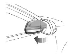
Rotate the knob to the middle position, and push the knob down. The door mirrors will be folded automatically. Pushing the knob downwards again will return the mirrors to their original position.
