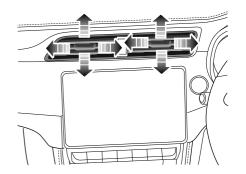
Slide the button in the centre of the louvres to the left or right to open or close the vent.
