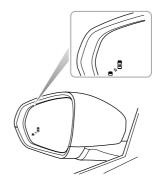
Note: The radar requires calibration on new vehicles or for vehicles of where a rear detecting radar sensor has been replaced. The rear detection radar sensors possess an automatic calibration function to compensate for installation error within a certain range. When the vehicle is running, the radar will automatically enter the calibration state. During the calibration process, the system will provide limited functions, and the alarm may be inaccurate. Upon
