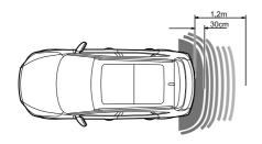
If there is an obstacle within 1.2m range from the rear sensors, the system starts to emit a beeping sound. As the vehicle moves closer to the obstacle, the beeps are transmitted more rapidly.
