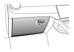
To open the glove box, pull the handle on the glove box cover (as indicated by the arrow).
