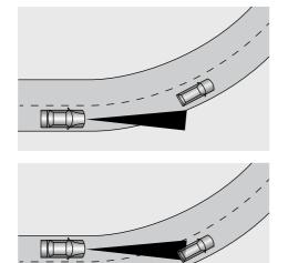
When turning at an intersection or following a vehicle into, or out of a curve, the adaptive cruise control system may
