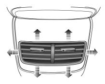
Slide the button in the centre of the louvres to the left or right to open or close the vent.
