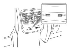
There are two USB ports located at the rear of the centre console, these provide a 5V power source as a power outlet.
