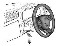
To adjust the angle of the steering column to suit your driving position:
