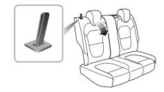
To increase luggage space, the rear seat backrest can be fully folded forward. When folding the backrest, first fully lower (or remove) all the rear seat head restraints, and then pull up the backrest unlock straps on both sides respectively and fold the seat backrests forward.
