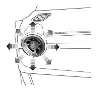
Rotate the centre thumb-wheel clockwise or anti-clockwise to open or close the vent.
