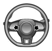
Press the horn button area on the steering wheel (as indicated by the arrow) to operate the horn.
