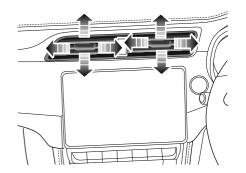
Slide the button in the centre of the louvres completely to the left or right to open or close the vent, adjust this button to direct the flow of air.
