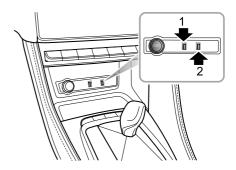
The 12V power socket is located under the shift control knob assembly in the centre console. It can be used as a power supply when the START/STOP Switch is in the ACC or ON/RUNNING positions when the blanking plug is removed
