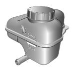
It is recommended that the cooling system should be checked weekly when the cooling system is cold and with the car resting on level ground. If the level is below the 'MIN' mark, remove the expansion tank cap and top up coolant, the level must not be higher than 'MAX' mark.
