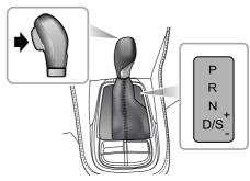
The automatic transmission is a 6 speed transmission.
