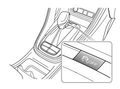
With the START/STOP Switch is switched ON/RUNNING, SCS and TCS will automatically turn on. And you can turn them off after the engine is started.
