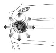
Rotate the centre thumb-wheel clockwise or anti-clockwise to open or close the vent. Toggle the centre thumb-wheel up, down, left or right to adjust the air direction.
