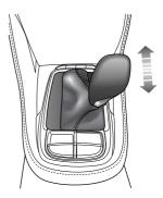
Move the shift lever toward "+" direction to upshift to next available high gear, move toward "-" direction to downshift to next available low gear.
