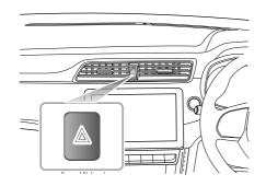
Note: Before you stop or slow the car in an emergency, always press the hazard warning switch. All the direction indicators will flash together to warn other road users when your car is causing an obstruction or
