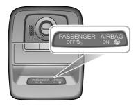
The passenger airbag status light is located in the roof mounted interior lamp assembly. The shape of the lamp assembly varies according to the configuration of the vehicle
