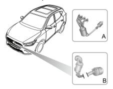
The exhaust system incorporates a catalytic converter and particulate filter (model dependant), these process possible harmful exhaust emissions from the engine into more environmentally friendly gases. Exhaust system layouts differ between engine derivatives. The 1.5L exhaust features (A). The 1.0T exhaust features (B).
