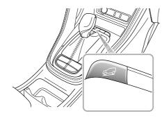
When the START/STOP Switch is switched ON/RUNNING, HDC system defaults to off. Use the switch function within the infotainment system to turn the HDC system on/off.
