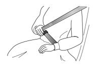
3 Insert the metal tab into the buckle until you hear a 'click',this indicates the seat belt is securely locked.
