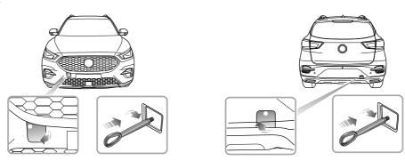
Your car is equipped with a removable towing hook, that can be used at the front or the rear of your vehicle. The towing hook is stored in the tool kit beneath the loadspace floor when not in use.
