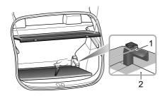
The rear parcel shelf is connected to the tailgate using straps and hooks. When opening the tailgate, the shelf will automatically be raised.
