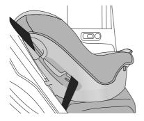
It is recommended that children should always be seated in the rear of the vehicle in a child restraint or restraint system, and fixed with 3 point, lap diagonal seat belts.
