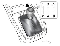
The manual transmission is a 5-speed transmission with 6 gears, which are: 1st, 2nd, 3rd, 4th, 5th, R (Reverse) respectively.
