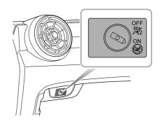
The passenger airbag disable switch is located inside of the glovebox, To disable the passenger airbag, insert the key and turn the switch to OFF position.
