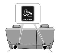
To fasten the Top tether strap of the child restraint system, route the tether strap under the head restraint and attach to the anchorage hook being careful not to twist the strap. If not using ISOFIX lower anchorages, using the seatbelt, complete the installation in line with the child restraint manufactures instructions.
