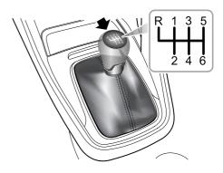
The manual transmission is a 6-speed transmission with 7 gears, which are: 1st, 2nd, 3rd, 4th, 5th, 6th, R (Reverse) respectively.
