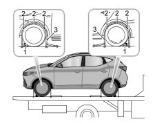
I Position the car on the trailer, apply the parking brake, and place the shift lever in N position (manual transmission), or in P position (automatic transmission).
