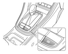
With the driver's seat belt fastened, the door closed and the engine running, press the auto hold switch to switch the auto hold function from Off to Standby state.
