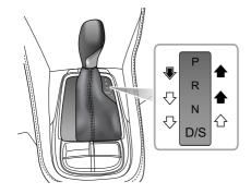
During the gear shift, operate the shift lever according to the instructions indicated by the following arrows:
