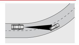
When turning at an intersection or following a vehicle into, or out of a curve, the ACC system may be unable to detect the vehicle ahead, even if it is in the same lane, it is possible the system may detect a vehicle in another lane.
