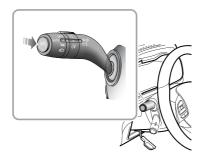
Having turned the lane departure warning system on in the infotainment display, press the button at the end of the indicator stalk switch (as shown above). The lane departure warning system will enter the standby or active state. The system defaults to the last selected state from when the START/STOP Switch was ON/RUNNING.
