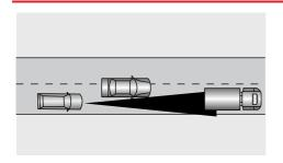
If the vehicle ahead changes lanes, but does not drive into the lane completely, the ACC system may be unable to detect the vehicle.
