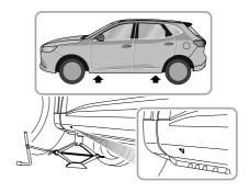
Turning the jack screw handle by hand, adjust the jack until the jack head fits snugly onto the flanging of the body. Ensure that the base of the jack is in full contact with the level ground.
