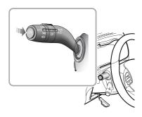
Having turned the lane departure prevention system on in the infotainment display, press the button at the end of the indicator stalk switch (as shown above). The lane departure prevention system will enter the standby or active state. The system defaults to the last selected state from when the START/STOP Switch was ON/RUNNING.
