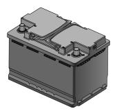
You can see the battery when you open the engine compartment. The battery is maintenance-free type, therefore there is no need to refill fluid.
