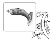
Having turned the lane keeping assist system on in the infotainment display, press the button at the end of the indicator stalk switch (as shown above). The lane keeping assist system will enter the standby or active state. The system defaults to the last selected state from when the START/STOP Switch was ON/RUNNING.
