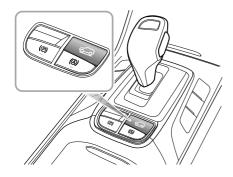
When the start/stop switch is placed in ON/RUNNING position, HDC system defaults to off. Press the button to turn on/off HDC system.
