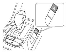
Note: Before you stop or slow the vehicle in an emergency, always press the hazard warning switch. All turn signal lamps and direction indicators will flash together to warn other road users when your vehicle is
