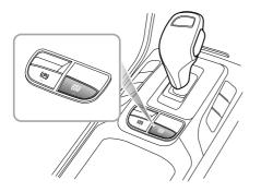
With the driver's seat belt fastened, the door closed and the engine running, press the auto hold switch to switch the auto hold function from Off to Standby state. With the brake pedal firmly pressed and the vehicle completely stopped, the auto hold function will switch from the Standby state to the Parking state.
