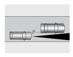
When driving behind a vehicle that is only partially overlapping your vehicle, 'A' in the graphic, the ACC system may be unable to detect anything.
