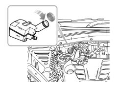
Note: Brake fluid will damage painted surfaces. Soak up any spillage with an absorbent cloth immediately and wash the area with a mixture of car shampoo and water.
