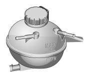
It is recommended that the cooling system should be checked weekly when the cooling system is cold and with the car resting on level ground. If the level is lower than 'MIN' mark, open the expansion tank cap of the cooling system and top up coolant, but the level shall not be higher than 'MAX' mark.
