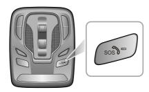
The emergency services call (eCall) system will perform a self-test when the ignition is turned ON. During a Self-Test the emergency services call (eCall) LED status indicator on the SOS button will flash quickly until completion. The LED status indicator will be illuminated solid if no system faults are present. The LED status indicator will be extinctd or
