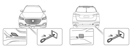
Your car is equipped with 2 towing eyes (located at the front and the rear of the vehicle), which are used for fitting the towing hook in the tool kit. The tool kit is placed beneath the loadspace floor. To fit the towing hook, remove the small cover set into the bumper, then screw the towing hook via the small hole into the threaded hole in the bumper beam (see illustration). Ensure the towing hook is fully tightened!
