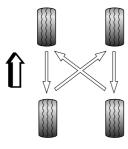
Note: Directional tyres (identified from the arrow on the tyre side) CANNOT be swapped from side to side.
