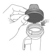
Check the washer fluid level every week. When the level of washer fluid is low, please top up the washer fluid as instructed. Please use the washer fluid recommended and certified by the manufacturer. Refer to 'Recommended Fluids and Capacities' in "Technical Data" chapter.
