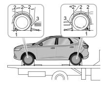
I Apply the parking brake, manual transmission places the shift lever in Neutral (N), automatic transmission places the shift lever in Park (P).
